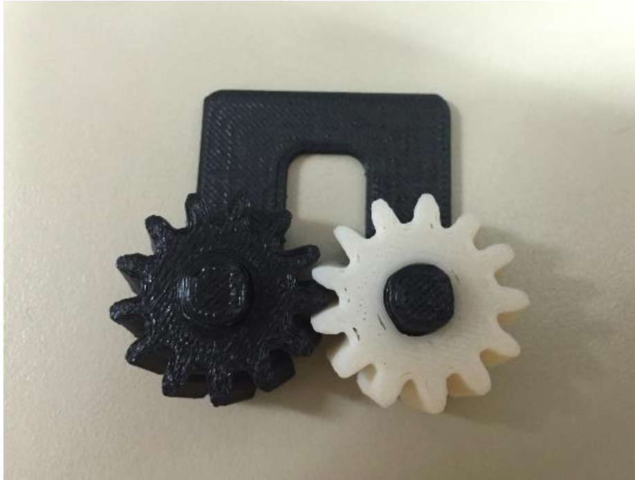
Figure 17: Two helical gears in action – made by 3D printing
